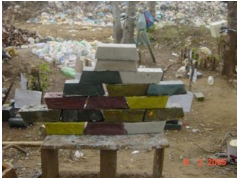
Transformation of plastic waste collected on the beach into construction bricks. Example of septic tank built with recycled waste bricks.
